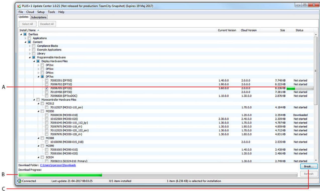
6. When installation is complete, the status of all newly installed items will be set to "Install Complete" and the Install button will have its original text back.
