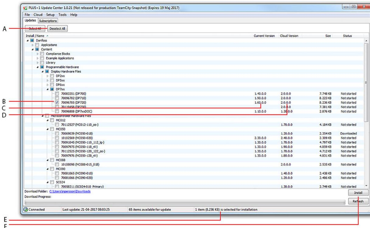
5. Make sure PLUS+1® GUIDE is not running and press Install to start the installation. The text of the Install button will change to Break... and the progress bars should start updating.
