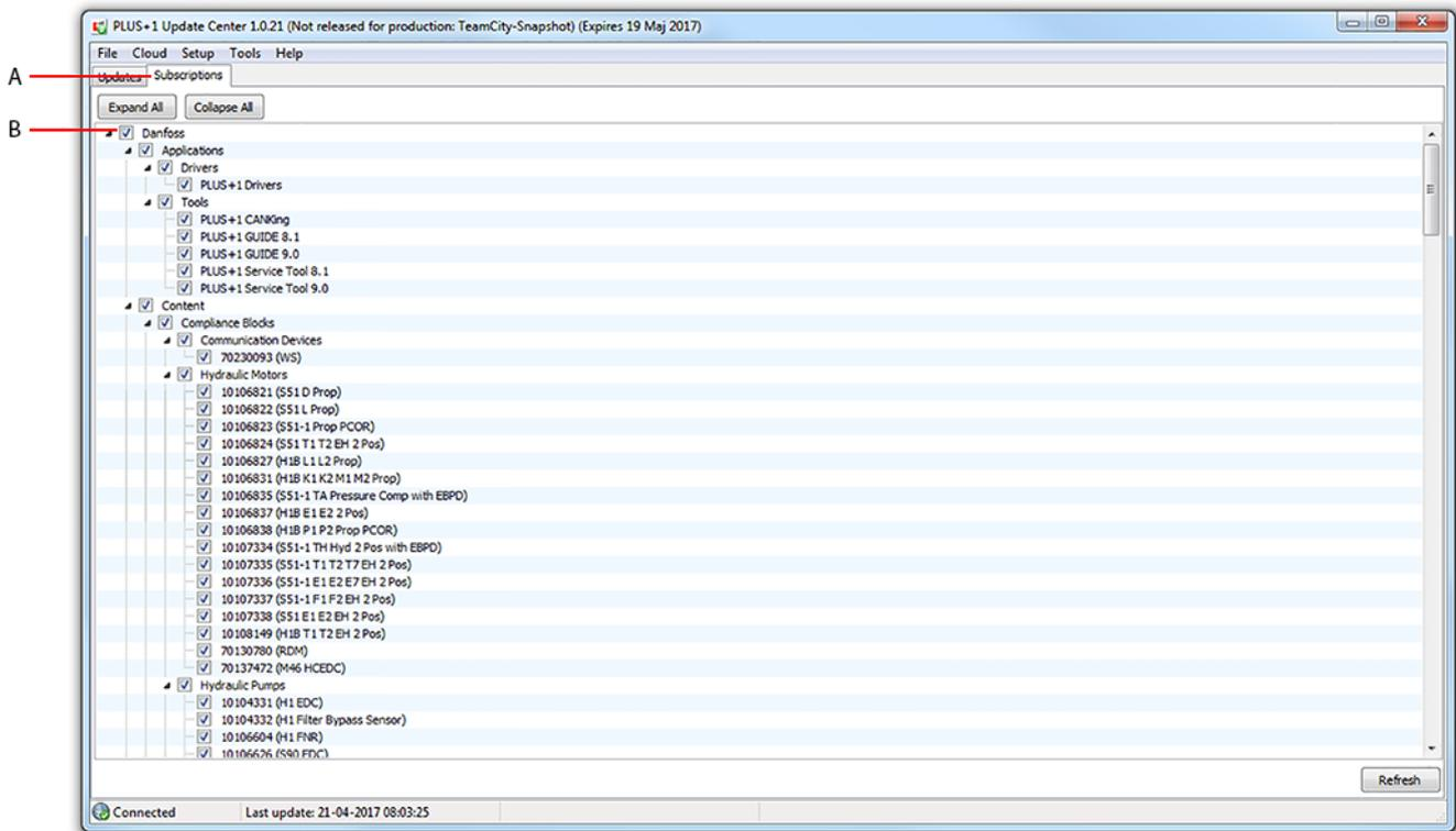
4. Go back to the Updates tab. Press “Deselect All” button in the Updates tab, then navigate to branch Danfoss/Content/Programmable Hardware/Display Hardware Files/DP7xx. In that branch, select 70096705 (DP720). If the latest version of that HWD is already installed it will not be visible in the Updates tab. For the purpose of this example, any other HWD could be used.
